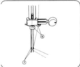
At guide **(6)**, pass one of threads to right guide and the other at left guide.
